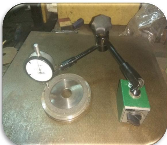
Fig 8 Brake Liner surface check [10]
